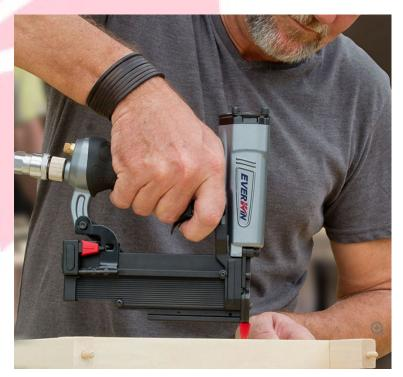
This size leaves a smaller indent in the workpiece compared to the 18-gauge, but with just enough holding power, excellent for more delicate work. As you go higher in gauge, the indents in the workpiece keep getting smaller which means you might keep on nailing without realizing that the tool had run out of fasteners. To combat this, a useful feature on our models is the dryfire lock out that prevents the tool from firing when there are no fasteners in the chamber.
